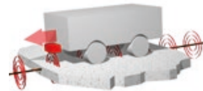
Inductive track guidance system
