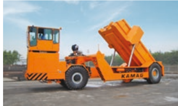
U-Frame Dumper: the hydraulic dumping device facilitates a dumping angle of min. 45°.
