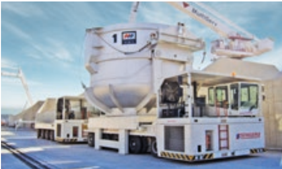
The steering is dimensioned to ensure that tyre wear is kept to an absolute minimum.
