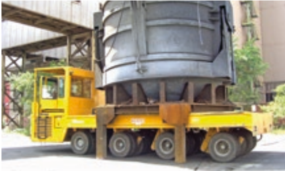
Scrap Basket Transporter for moving scrap materials in a steel plant.
