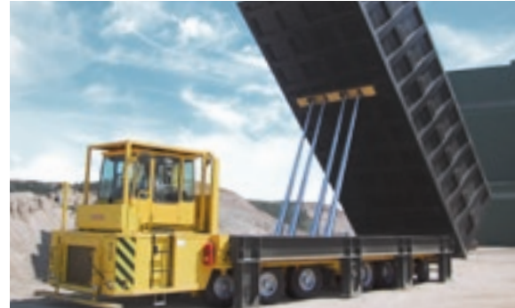
The swap body and generous dumping angle up to 60° ensure complete emptying during the handling of scrap materials thus providing yet another advantage.
